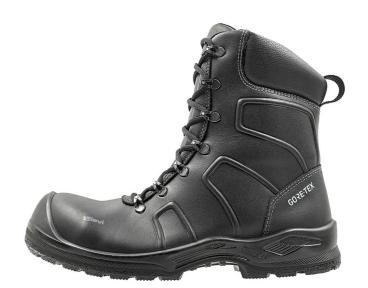
The GT 25+ is a safety shoe with GORE-TEX lining for varied conditions. GORE-TEX is a waterproof and breathable microporous film laminated onto the lining of the footwear. The foot is protected by a composite toecap and penetration-resistant steel midsole. The upper is made of durable top-grain leather. Zip fastening on the side and lacing on the top. DUAL Comfort insoles for added comfort.
