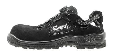
Durable safety footwear with a composite toe cap and a penetration-resistant steel midsole. Thanks to the 3D-dry® lining and the vents on the upper, the shoes are breathable and comfortable to wear. The FlexEnergy® heel component absorbs kinetic energy, more than 55% of which is returned to the wearer. The BOA® Fit System lacing mechanism offers greater comfort. Antistatic and ESD approved.
