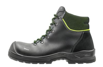
Lace-up ankle boots made of durable PU-coated leather with composite toecaps and penetration resistant steel midsoles. Polyurethane soles are resistant to oil and a number chemicals and absorb shocks effectively. Breathable and structured insoles and 3D-dry® lining improve ventilation and make the boots comfortable to wear. ESD-approved.
